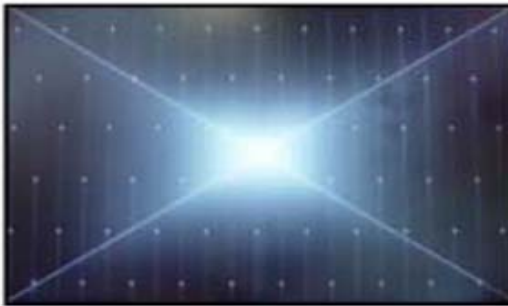
Solder defect, Short/Crack
